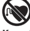
**Keep the laser spirit level away from cardiac pacemakers.** The magnets (11) generate a field that can impair the function of cardiac pacemakers.
